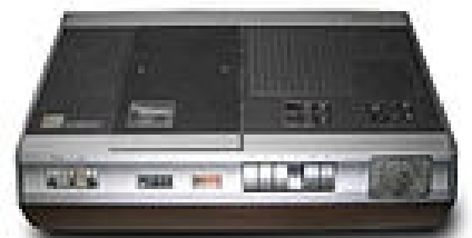
A Philips N1500 video cassette recorder.
